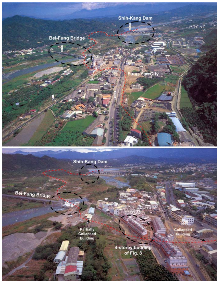
Fig. 17 Chelungpu thrust fault, Chi-Chi, Taiwan 1999 earthquake—Fung-Yan City. From bottomright to top-left: The fault rupture, of about 7 m of upthrust, passed through Fung-Yan City causing complete collapse of one building (the details of which are not known), substantial damage to three other buildings (shown in detail in Fig. 8), partial collapse of a light 1-story structure, collapse of two spans of the Bei-Fung Bridge, and failure of the Shih-Kang Dam (photos adapted from Hwang 2000 )
